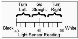
So now if the light level is less than 43 we want the robot to turn left. If the light value is between 44 and 47 we want it to go straight (zoom zoom). If the light level is greater than 47 we want to turn right. This can be easily be implemented in Mindstorms NXT-G with a switch (yes/no) within a switch. You actually only have to do two tests not three.
