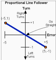
In the above graph I have shifted the axis by converting it to an error scale. Since the line now crosses the Y-axis at zero that mens b is is zero and the equation for the line is a bit simpler;
