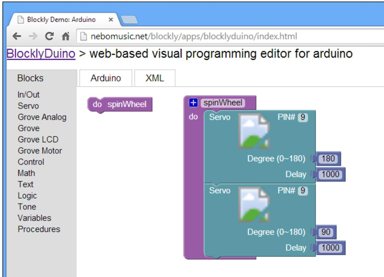
8. Copy the code from the Arduino tab to the Sketch program and download to your Arduino. The wheel on the servo should turn and stop.
