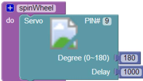
6. We want the wheel to stop. So, place another Servo block in the spinWheel procedure. Set the PIN# to 9, Degree to 90 (to stop), and the Delay to 1000.
